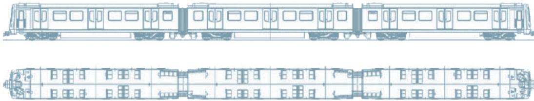
One train consists of three cars in the configuration MC1-M-MC2. The cars at the front and at the rear are motorized and equipped with a driver's cab (MC). The middle car is motorized without a driver's cab (M). The total train length is 54.34 m with a maximum transport capacity of 678 passengers. The maximum speed is 80 km/h.
